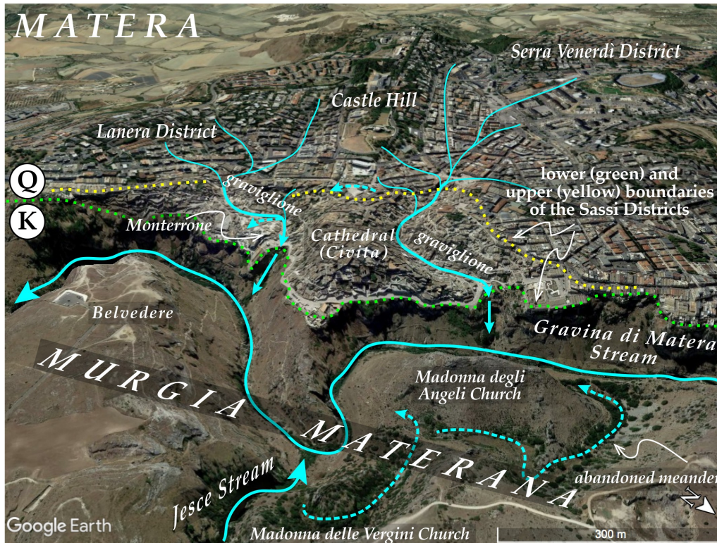
Fig. 2 - Aerial view of the Murgia Materana and the Matera town with some of the toponyms used in the text. The green dotted line indicates the boundary between Cretaceous (below) and Quaternary (above) carbonate rocks; the yellow dotted line indicates the boundary between Quaternary carbonates (below) and Quaternary clay deposits (above). Top of the hills ( Lanera , Castle , and Serra Venerdi ) are characterized by sand and gravel. The Sassi Districts were dug in the Quaternary carbonates (i.e. the Calcarenite di Gravina Formation). Base image by Google Earth.
